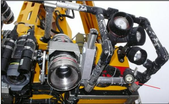
Figure 6. Canadian Scientific Submersible Facility - ROPOS ROV before an evaluation dive with DSPL's LED-MultiSeaLite® (red arrow), and other lights. [Photo by Reuban Mills, ROPOS]
